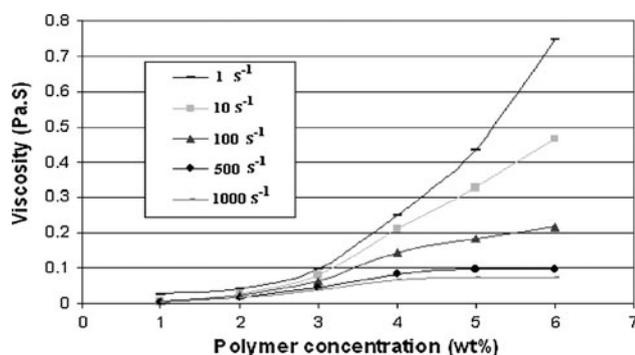
**Fig. 1** Viscosity as a function of concentration and shear rate for aqueous A1(L1) samples analysed at 20 °C using parallel plate rheometry
