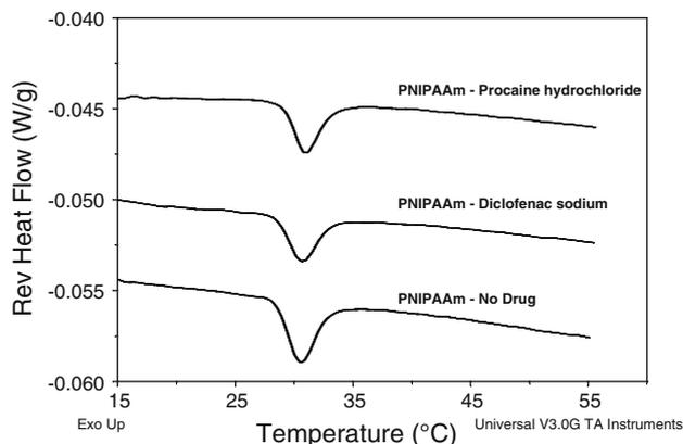
**Fig. 2** LCST endotherms of 3 wt% PNIPAAm homopolymer before and after drug incorporation
