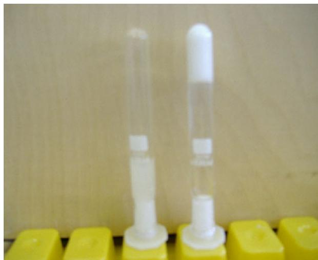
**Fig. 3** Visual illustration of thermoreversible A1(L1) copolymer at 6 wt% in pH 6.8 buffer media: sol at room temperature (*left*) and gel having been submerged in a water bath at 44 °C (*right*)
